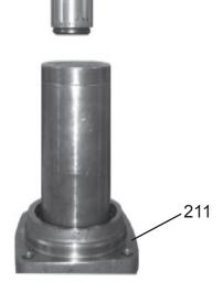
Push on the bearing ring (item 470) in the bearing housing (item 211) with a press. Use a tube to match the outer diameter off the bearing ring.
