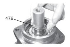
Push on the Bearing (item 470) with a press until correct preload is achieved. Install the spacer washer (item 476).
