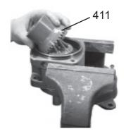
Install the cylinder barrel (item 411). Ensure correct timing. (Marking, punch mark)
